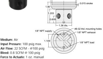
**Mounting:** Mounting holes provided; optional Bracket Kit #2010-50 provides additional mounting versatility; valve available with anodized color buttons
